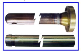
The lance tube is 3.5" chrome moly tubing with SS head assembly. The flange is a forged & machined one-piece design made integral with the lance for durability and safety. Nozzles can be high impact or flush ground. The lance is indexed during travel to allow for an infinite number of cleaning helix paths improving cleaning coverage and reducing erosion.
