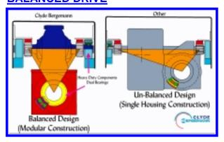
The dual rack-and-pinion drive has been developed using a "Balanced Design" concept. All major components such as the poppet valve, feed tube, traveling carriage and lance
