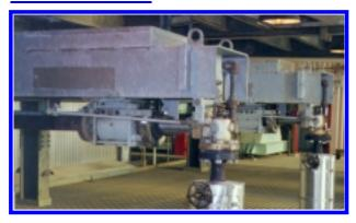
To improve the maintainability, the RS provides easy access to all essential components. For example, the large top opening allows removal of the gearbox within 30 minutes, compared to several hours with competitive sootblowers. Other components such as valve operating mechanisms, and proximity switches are externally located to the housing for better access.
